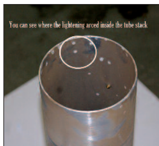
Missing / melted finger stock that holds tube in place and clamp missing as well.
